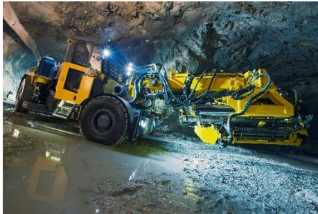
An Atlas Copco Simba ME7 C drilling rig
