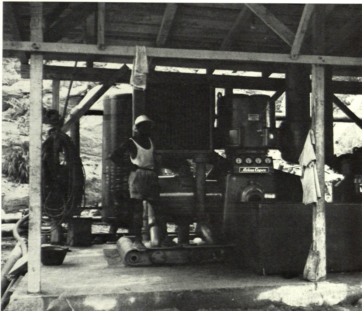
Above: Supplying air power to work for hydro power at Akosombo, site of the main dam in Ghana's Volta River Project. Eight of these ET6 compressors are included in the Company's equipment used by the Italian contractors Impregilo.
