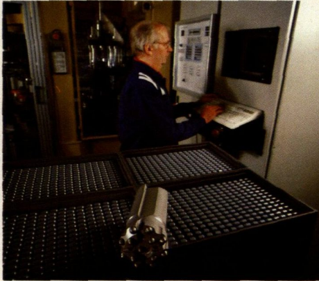
Production of cemented carbide for the rock drilling tools.
