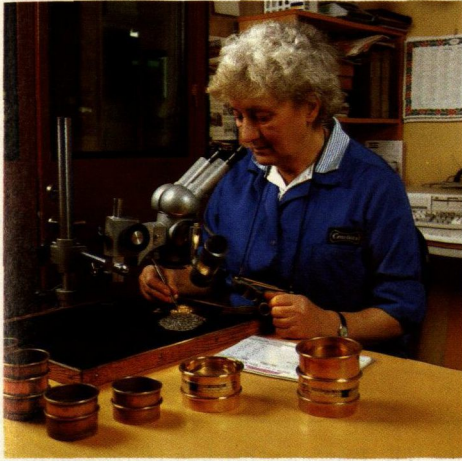
Sorting of diamonds for mounting on a diamond drill bit at the Craelius plant in Märsta, Sweden.
