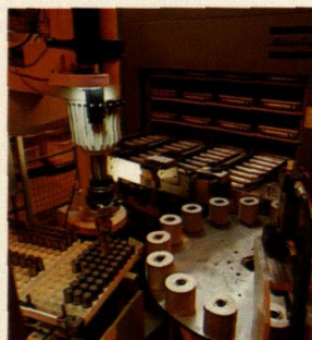
Cover: Automatic assembly of up to 60 different types of pneu- matic tool motors at the Atlas Copco Tools' plant in Tierp, Sweden.
