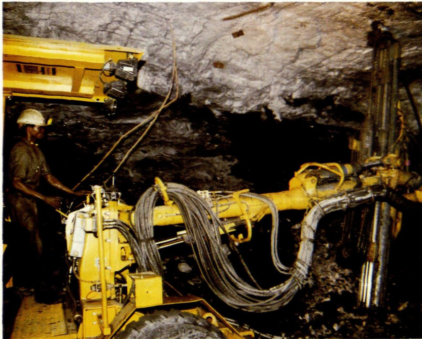
A modern hydraulic drilling rig for the mining of gold in Ghana.
