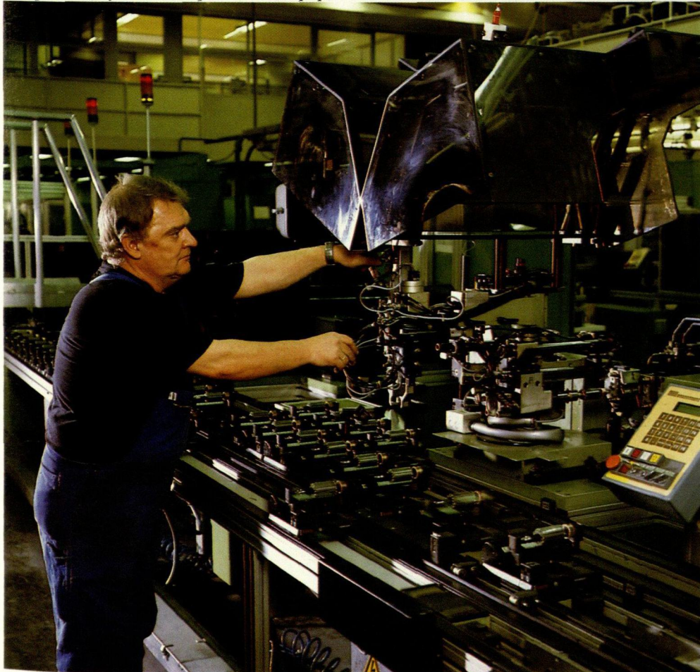
A winding station in the new, wholly automatic assembly line for rotors at the electric tools plant in Winnenden, Germany.
