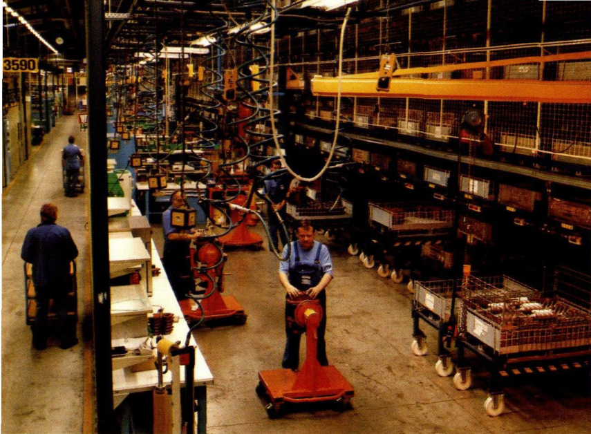
The assembly of complete compressor elements is conducted with optimal efficiency through automated material flows.
