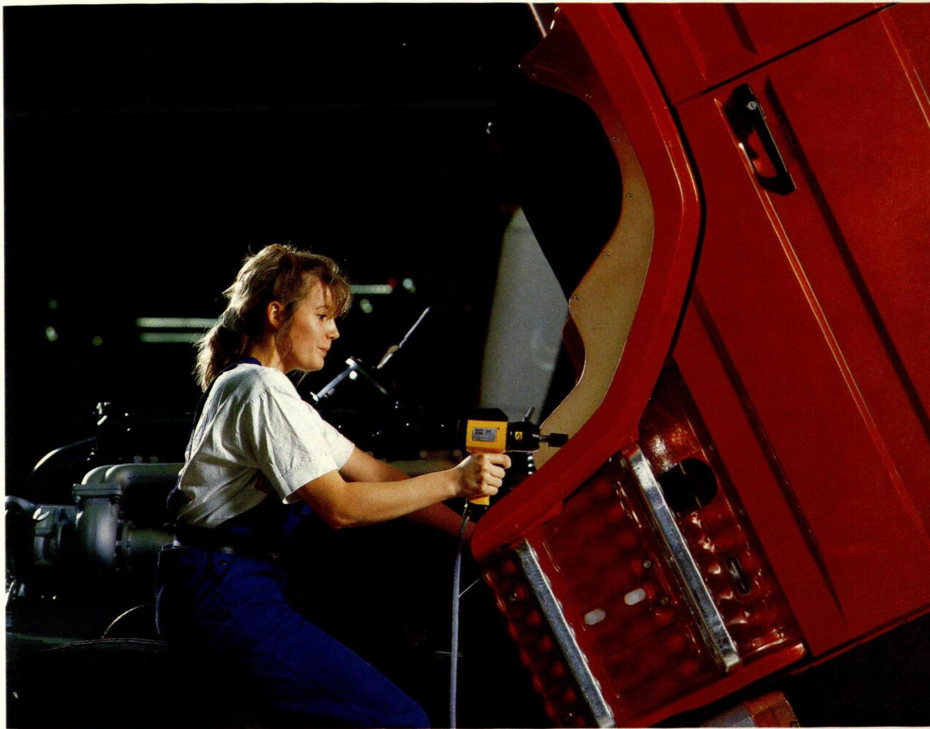
ErgoPulse, a new generation of pulse nutrunners with excellent ergonomic properties, was introduced during the year.
