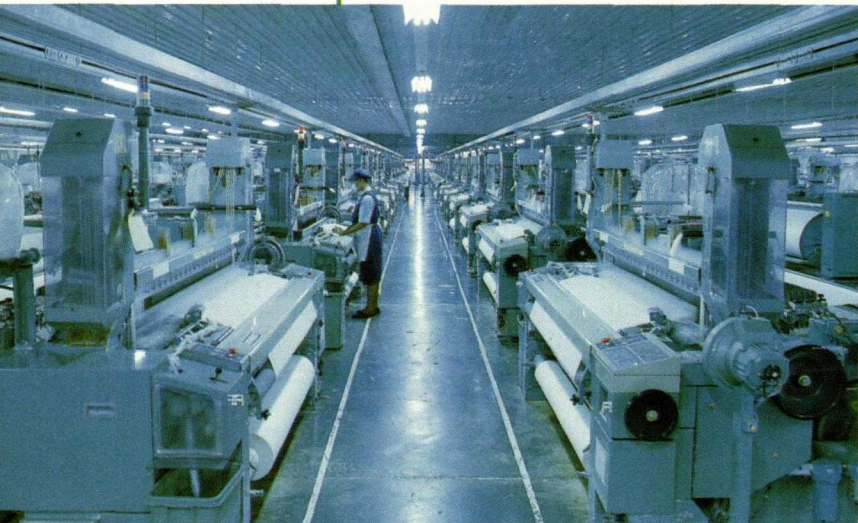
The use of compressed air jets in woven textiles production has resulted in increased productivity and improved product quality.
