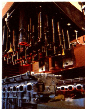
Cover illustration: An assembly system with 49 spindles for tightening of engine bolts. MACS, an advanced, com- puter controlled system, is re- sponsible for quality assurance.
