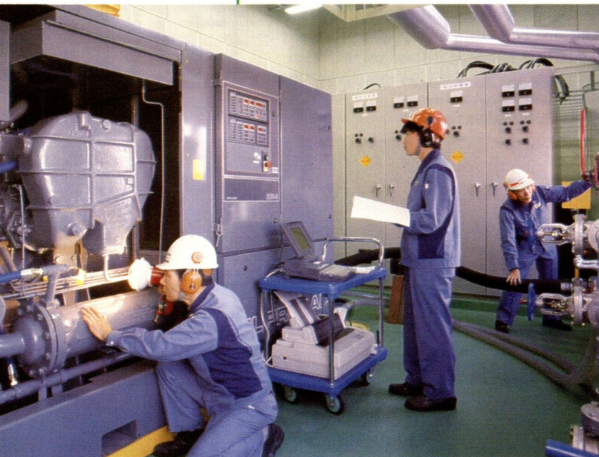
Final testing and quality control of oil-free compressors at the Atlas Copco KK's plant in Japan.
