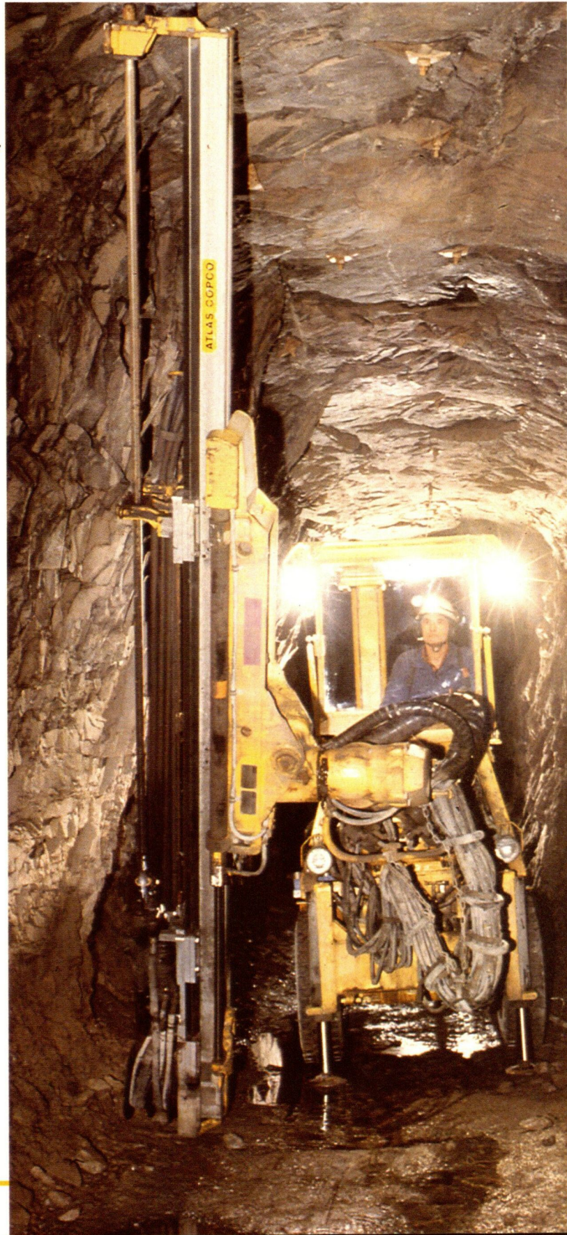
A new type of drilling rig for the mechanized extraction of narrow ore-bearing strata was launched during the year.
