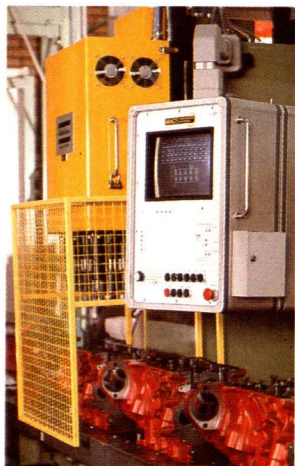
An increasingly large part of Atlas Copco Assembly Systems' sales stem from the needs of customers to document production-related quality. This is accomplished through the connection of tightening-spindles to advanced monitoring systems.
