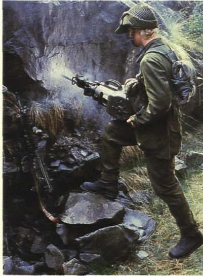
Several large military orders for the easily handled, fuel-powered drills/breakers, Cobra and Pionjär, contributed to the sharp increase in sales.
