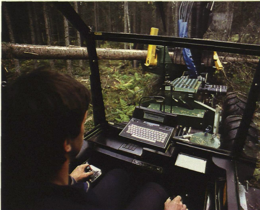
Logging machines are increasingly equipped with electro-hydraulic control systems from Monsun-Tison. Productivity is improved via these systems and felling operations can be controlled with just two mini levers. The operator is also provided with a more ergonomic working position.
