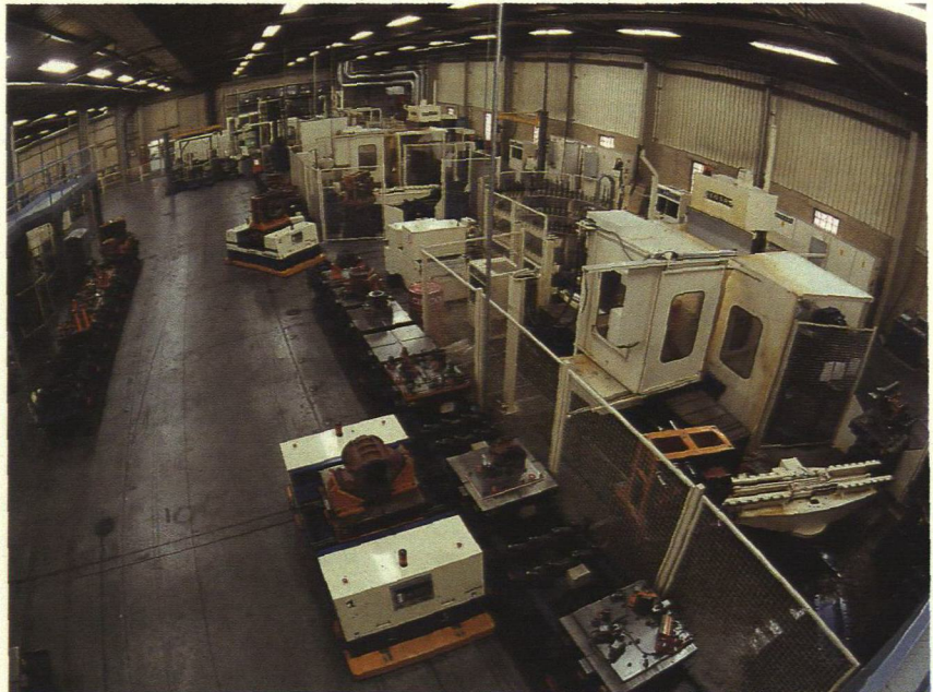
A flexible manufacturing system in operation at the Airpower plant in Antwerp, Belgium, has reduced production time for components considerably.
