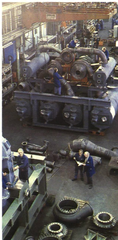
Assembly of a six-stage turbo compressor at the ACT plant in Cologne, West Germany. Standardization of assembly techniques for the various components has resulted in considerable time savings in production.
