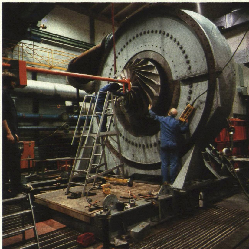
Assembly at the Cologne plant of a single-stage centrifugal compressor for a purification plant in Chicago, U.S. Compressed air from the compressor is used for oxygenization of the waste water.
