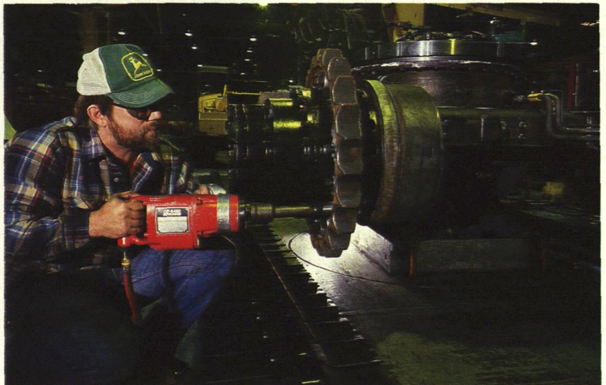
Chicago Pneumatic is recognized as one of the leading suppliers of pneumatic tools to industry in the U.S. Deliveries to John Deere include nutrunners for assembly of drive wheels.
