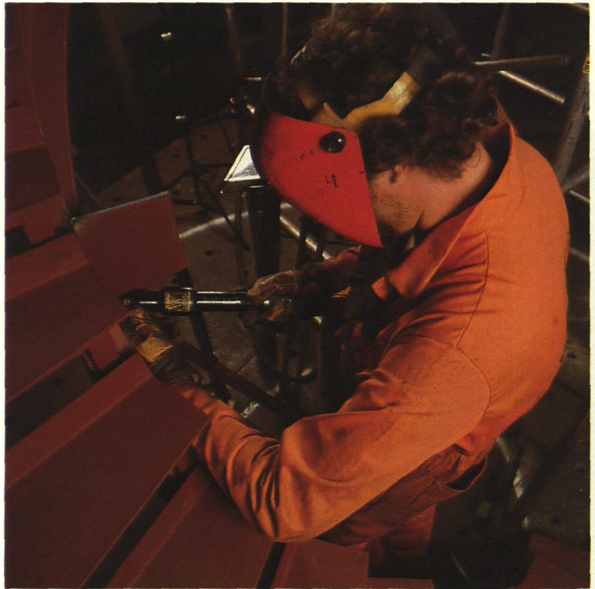
Ergonomically well designed tools are of greatest importance to the user. A chipping hammer, part of the Ergoline tool series from Atlas Copco Tools, is used at the Mälars Shipyard in Stockholm.
