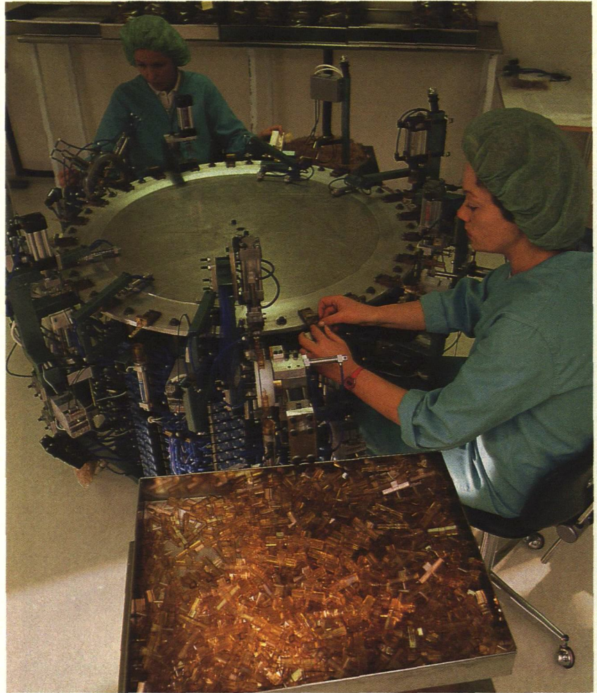
The assembly robot at the J S Medical factory in Husqvarna, Sweden, is controlled by a pneumatic control system from Monsun-Tison, who also delivered the compressed-air cylinders. The robots assemble disposable items used in medical care.
