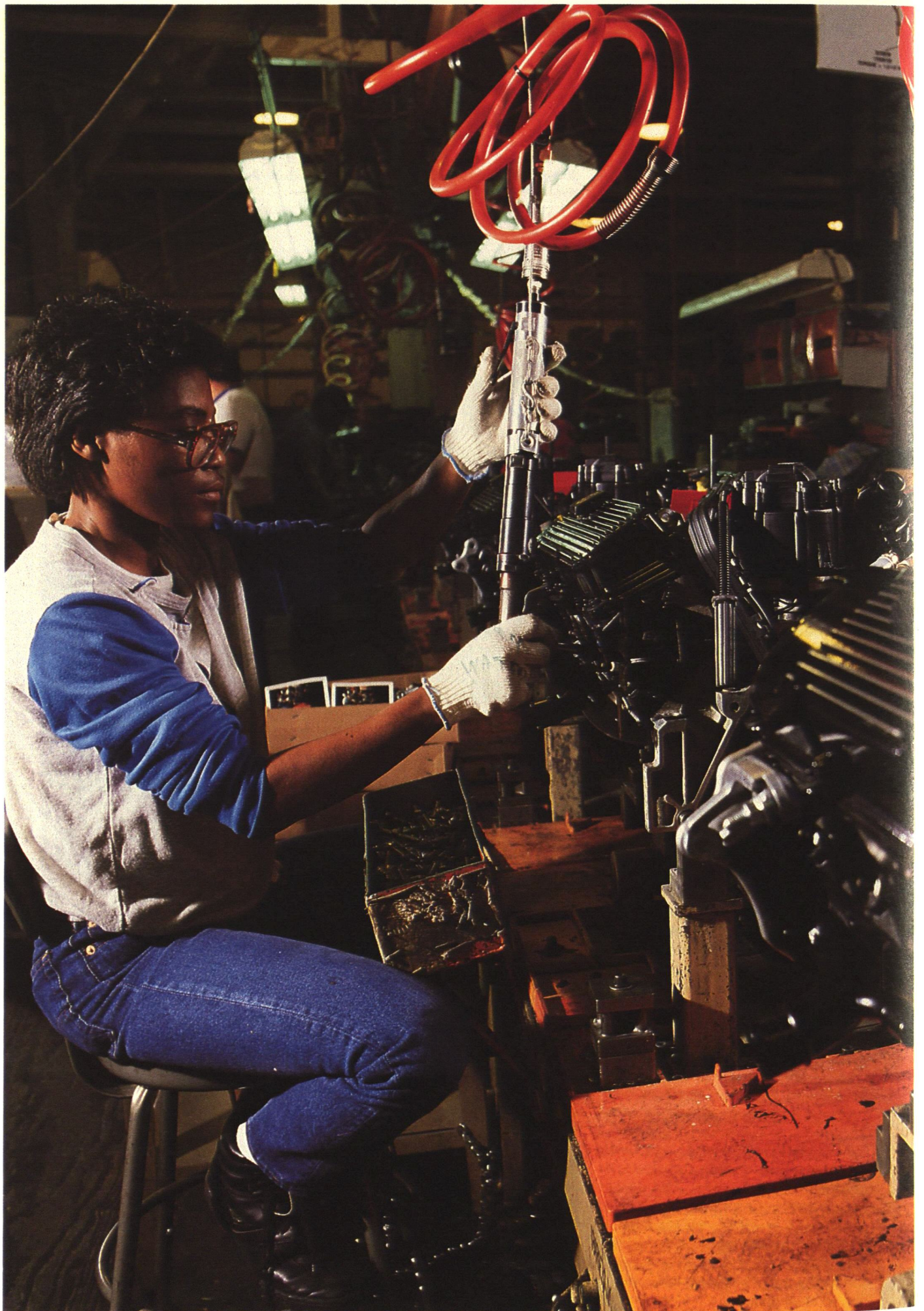
Leading automobile manufacturers use Atlas Copco's torque control nutrunners because of their exceptional accuracy. Shown is spark plug installation on an V8 engine final assembly dress line at a U.S. automobile plant.
