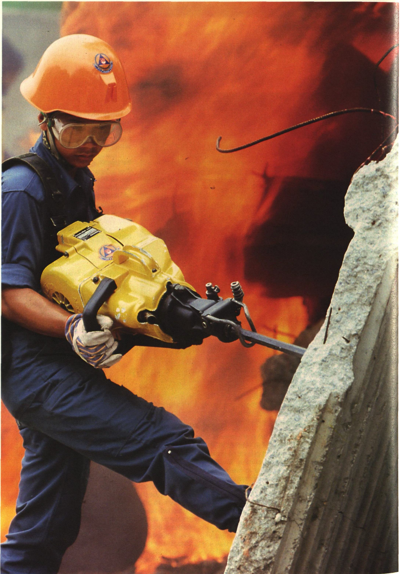
During 1986, Singapore's civil defense forces purchased a large number of Pionjär fuel-powered combination drill/breakers for use in rescue operations.
