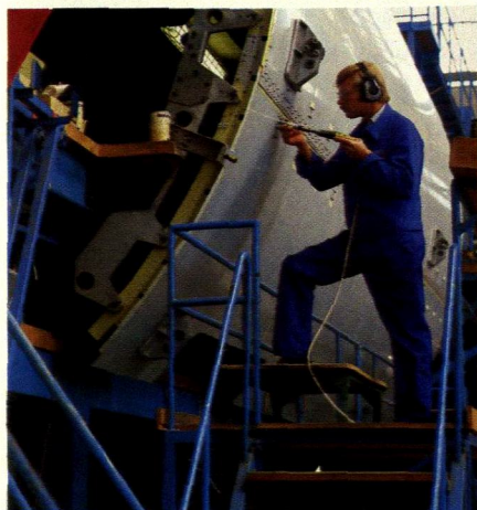
Atlas Copco's ergonomically designed tools for riveting, drilling and screwdriving are used frequently in aircraft production, where high demands are made on personnel and equipment. Picture shows screwdriving at an aircraft plant in West Germany.
