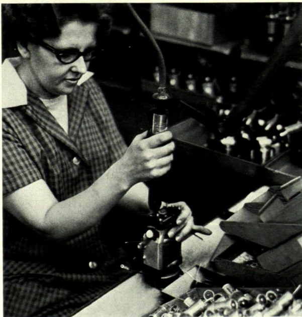
One of the new LUF 11 series of air-powered screwdrivers used in an Electrolux assembly shop for electric motors.
