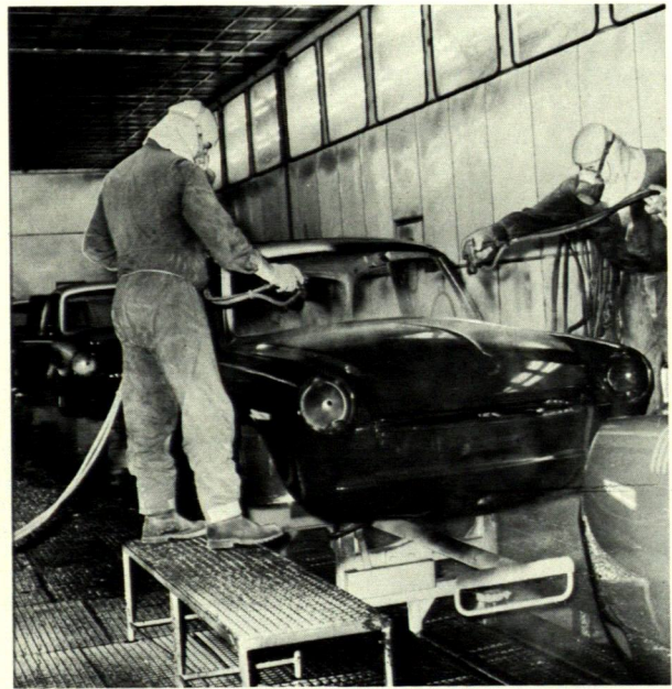
High-capacity Atlas Copco spray guns used for applying finishes at the Wolfsburg plant of Volkswagenwerk AG.
