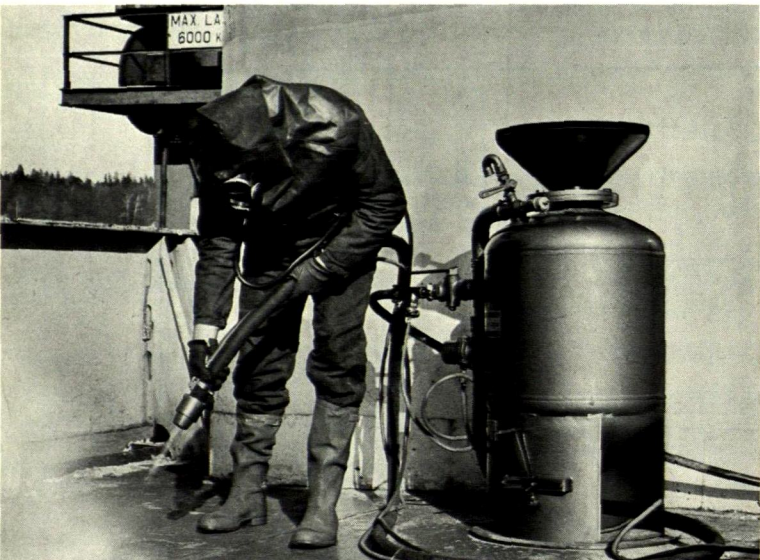
A new blast-cleaning unit tackles deck-rust on board ship.
