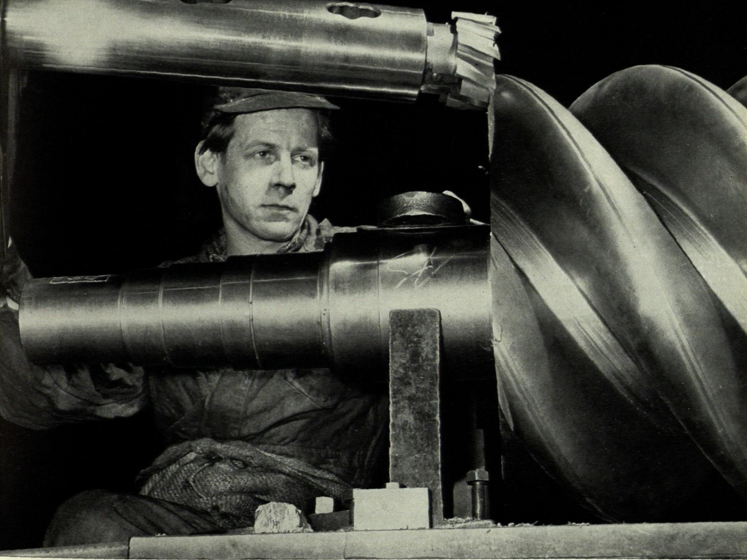
These industrial photo studies show something of the work carried out at the various production plants in Sweden. (Above) Cutting the screws for an Atlas Copco rotary screw compressor is a feat of engineering precision. In the final stages of cutting the tolerances are down to 0.05 mm.
