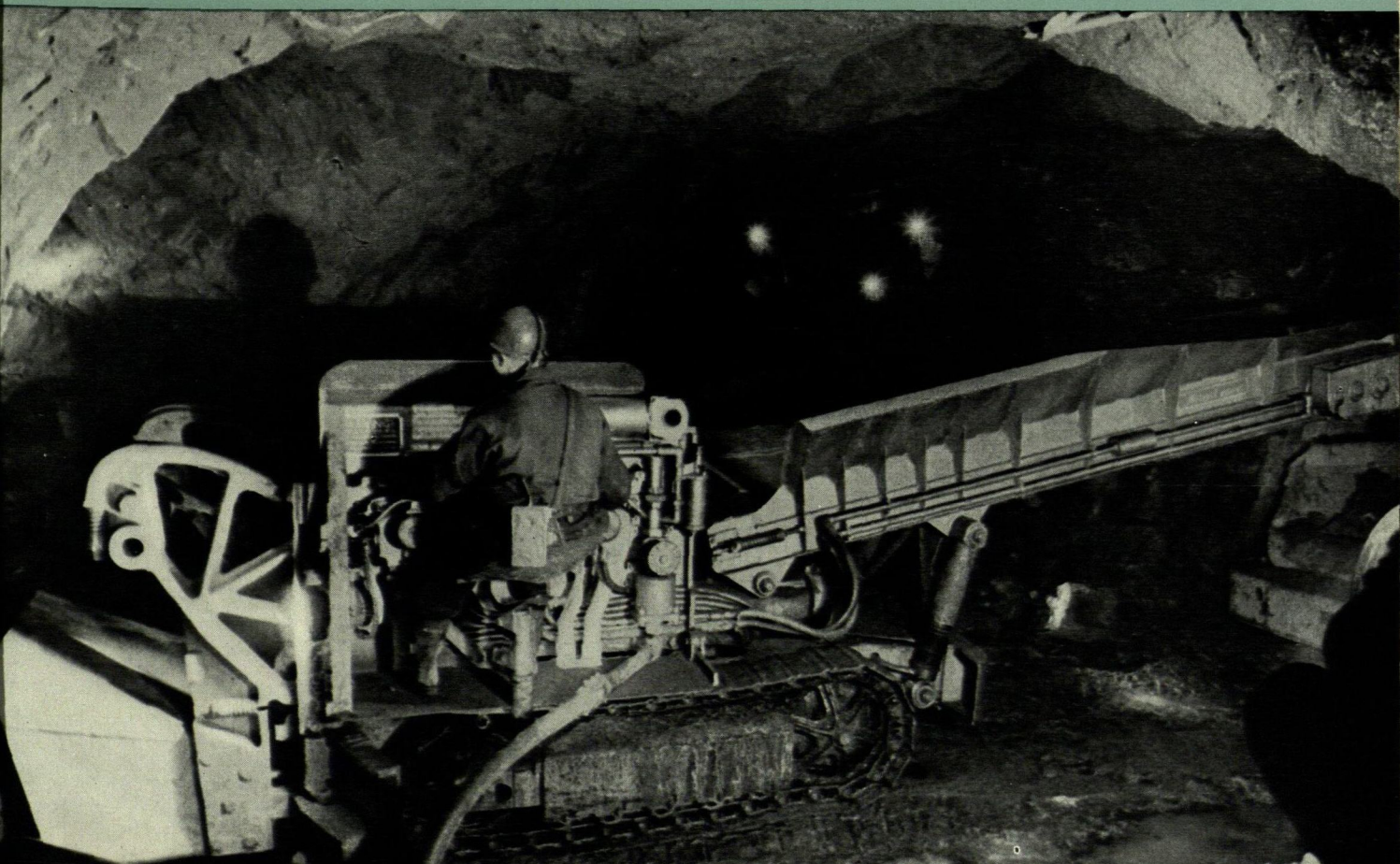
The track-mounted loader LM 500 in operation in Kiruna, Sweden, which is the world's largest underground mine. This machine can muck out 80 cubic yards of broken rock per hour.
