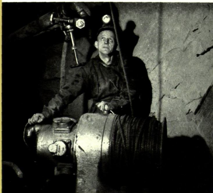
Avos manufacture chiefly pneumatic loaders, winches and hoists. The above photograph illustrating a pneumatic winch was taken in a Swedish mine.
