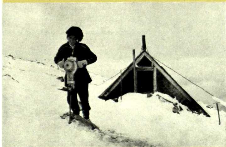
Below: During the summer of 1956 test drillings were made with satisfactory results with the new "Cobra" motor drill in the Swedish and Norwegian mountains and also in the Alps. The illustration shows the machine at work outside the but at the top of Mt. Kebnekajse, Sweden.
