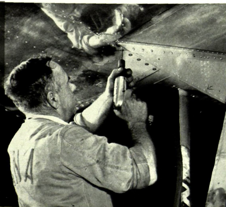
Injector's production comprises mainly pneumatic tools. The picture shows a screw-driver made by that company being operated at the Australian National Airways in Melbourne.
