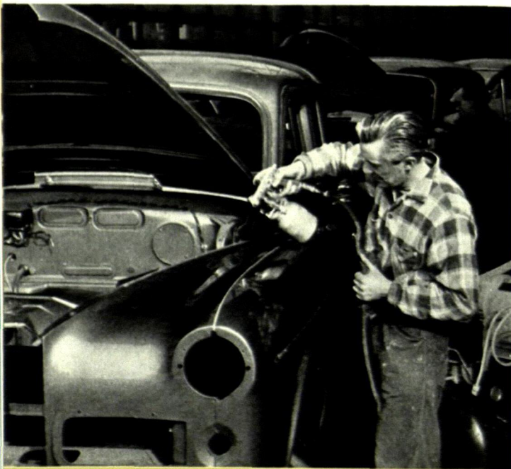
The principal products of the Eccoverken works are paint spraying equipment and small compressors. The illustration shows paint spraying with a spray gun, type Ecco 307, at the British firm of J. C. Beadle (Coachbuilders) Ltd.
