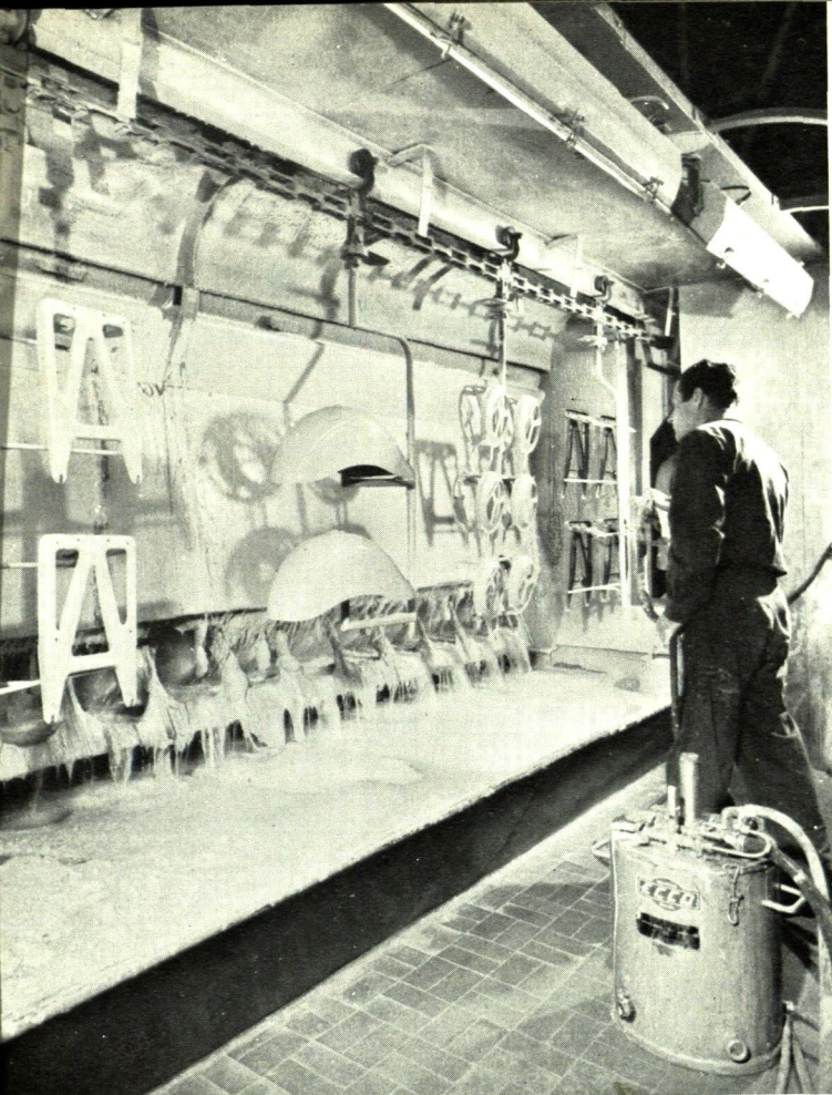
AB Eccoverken manufacture such articles as paint spraying equipment and small compressors. The above photograph was taken at the Vespa factory, Piaggio & C., Genoa, and shows an Atlas Copco hot-spraying unit being used to spray scooter components.
