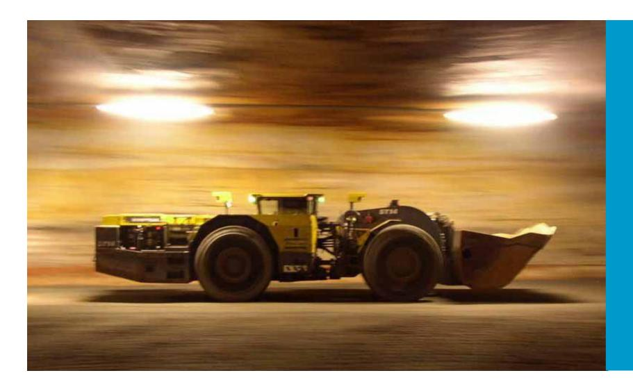
14 ton loader operating in a 10 ton loader sized drift
