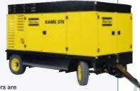
compliant with the European Outdoor Noise Directive 2000/14/EC, which means that units can run in the vicinity of hospitals, schools, and residential areas, even at night. Furthermore, the compressor frames are totally sealed to prevent potential leakage of oil and other liquids, and all engine types are compliant with Tier II/Stage II exhaust emission standards in both the United States and Europe.
