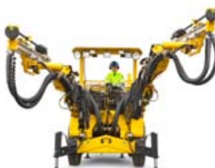
Two-boom face drilling rig
