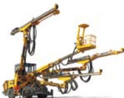
A three boom tunneling drill rig with a mechanized rod handling system for improved safety
