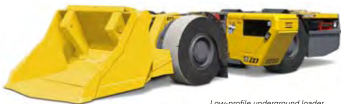
Low-profile underground loader
