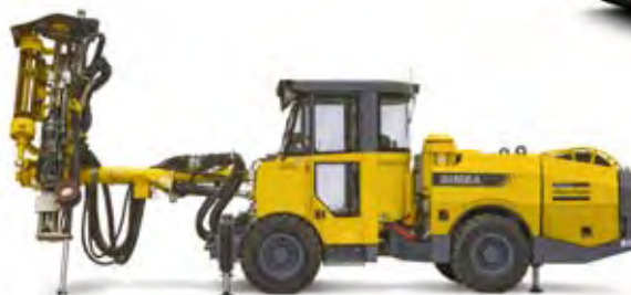
Production drill rig for underground mining
