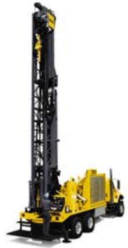
Deep hole surface drilling rig (max 1 500 m)
