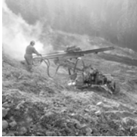
ROC 600 with separated rotated rock drill BBE 57 predecessor ROC 600 was the first AC crawler drill, introduced in 1964.
