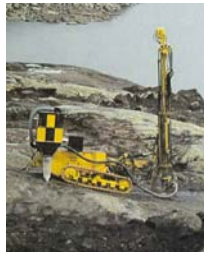
ROC 810H The first Atlas Copco hydraulic crawler drill rig, introduced in 1977.
