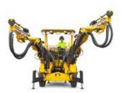
Two-boom face drilling rig
