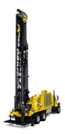
Deep hole surface drilling rig (max 1 500 m)
